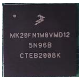
Images of the Freestyle Libre 2 processor(s) in the sensor and handheld receiver.
